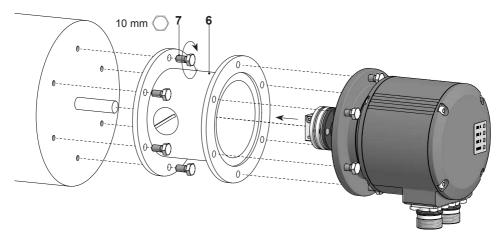
The encoder must be mounted with cable connection facing downward and not exposed to water.
